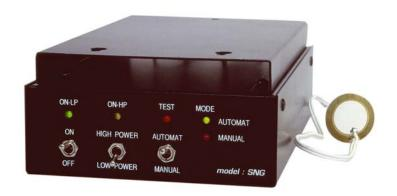
Piezoelectic elements are normally stuck on the window glass or installed on the room wall. Very efficient transfer of audio frequency noise vibrations ensures much higher noise on the target surface then any vibrations produced by conversation in a room. Any listening device picking up the conversation from the window or wall is disabled including the ultimate long range laser system which is badly affected even if focused on an object in a room because of Doppler phase noise modulation.
